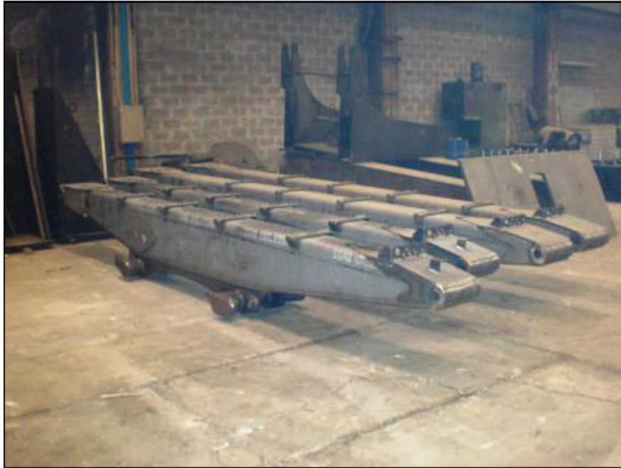
Boom in weldox 700
